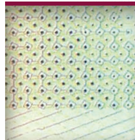
Line width modulation Lines with different line widths protect documents against professional counterfeiting
