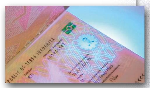
The transparent window can be considered a security feature as it is, but it opens space for placing other security features. The window provides a central position for placing a laser engraved secondary photo of the bearer that can be seen on both sides of the data page.
