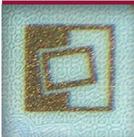
Optically variable print combined with up-converting feature
