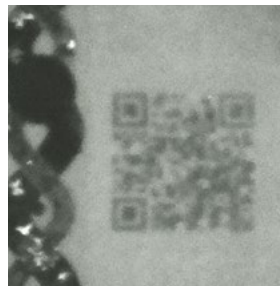
invisible, IR absorbing barcode
