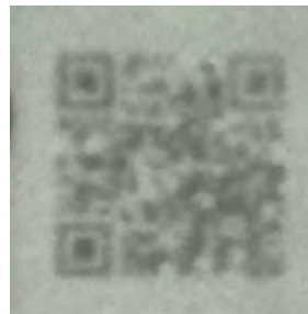
invisible, IR absorbing barcode
